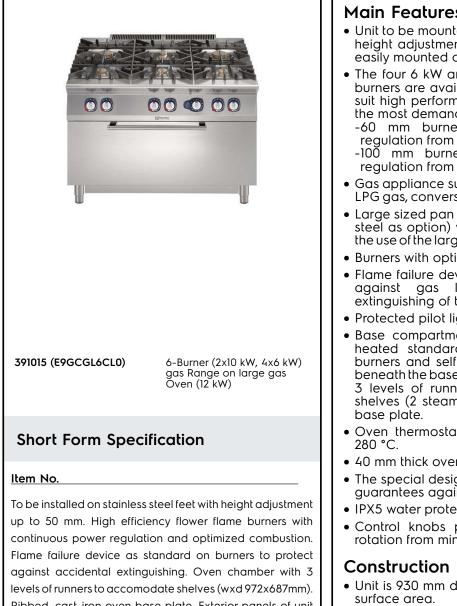
Ribbed, cast-iron oven base plate. Exterior panels of unit in stainless steel with Scotch Brite finish. Pan supports in heavy duty cast iron. Extra strength work top in heavy duty 2 mm Stainless steel. Right-angled side edges to allow flushfitting junction between units.
